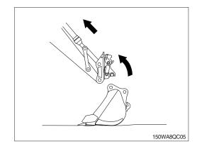
(8) Move the arm (1) and raise it until hook engages the upper (2) pin or interface of attachment.
